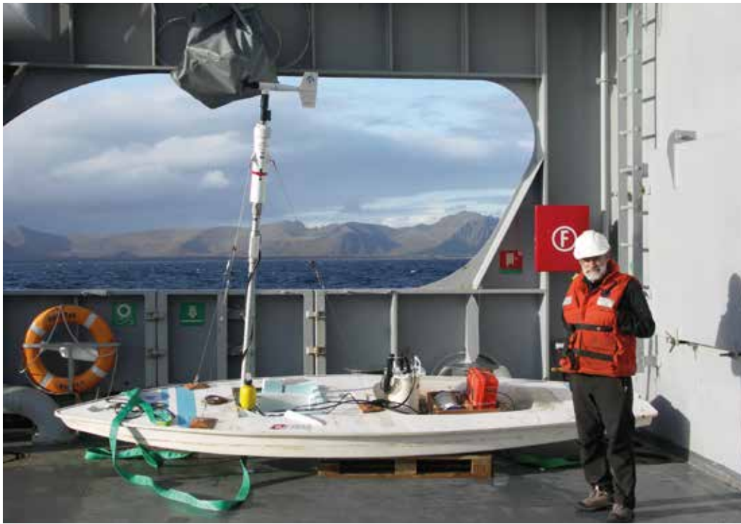
Art outfitted a sailboat for drift experiments with a wind-monitoring system, a current meter to measure the sailboat's drift, and beacons and straps to help recover the boat Credit: Øyvind Breivik, Norwegian Meteorological Institute
